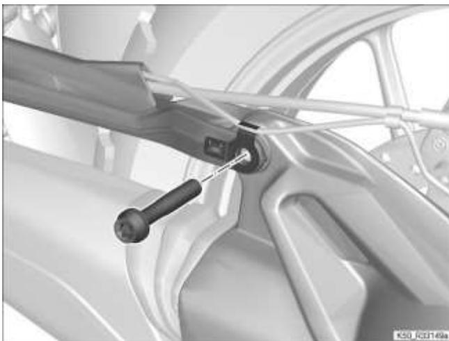
Since the existing screw is being re-used, it is essential to clean the screw as well as the thread in the differential, and use **Loctite 2701** - PN 33 17 2 331 095 when re-installing.
